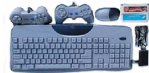
Figure 1: Typical keyboard-style TV-computer with working mouse, game-pads, and game cartridges
